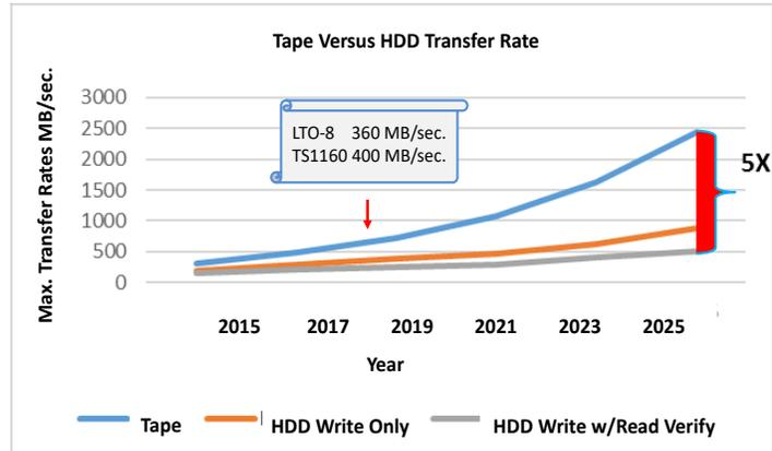
Note: Multi-channel head technology enables faster transfer rates in tape drives. Disk drives use a single active channel.
