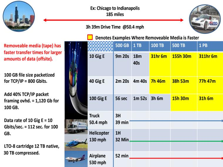
Removeable media (tape) has faster transfer times for larger amounts of data (offsite).
