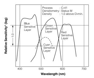
Sensitivity equals the reciprocal of exposure (J/cm²) required to produce a specified density.
