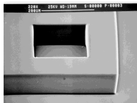
100 µm via in 40 µm softbake film
