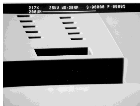
Via mask in 40 µm softbake film
