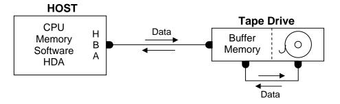
Today's drives are designed to operate in a streaming mode, not stop-start.
