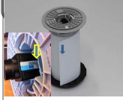
Slide the grey flange onto the spindle until fully pushed into the paper core. The number on the Spindle and the Paper Size match (8 inch paper shown)
