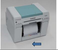
5. Carefully push the roll paper feeder into the printer.
