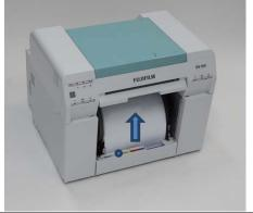
Carefully roll the paper back into the printer to take up any slack. Check that the blue paper light remains on.
