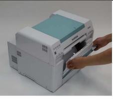
7. Insert the bottom section of the scrap box and then push the top section into place.
