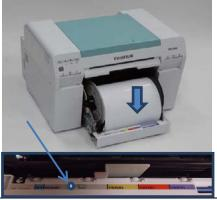
Insert leading edge of the paper into the feed slot until the blue paper light turns on.
