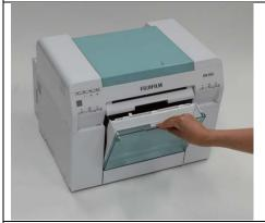
Remove the paper cuttings scrap box, by pulling top section forward and lifting it out. Make sure to empty and discard cuttings from the box.
