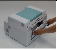
16. Insert the bottom section of the scrap box and then push the top section into place.
