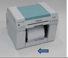
14. Carefully push the roll paper feeder into the printer.
