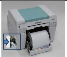
Load spindle unit in the roll paper feeder. Check that shaft of spindle fits into bearing as shown.
