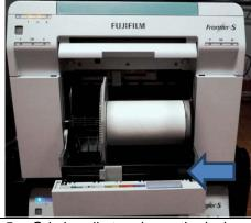
Grip handle to release the lock, then pull out the paper roll feeder. Remove the paper spindle and empty core.
