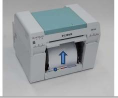
Carefully roll the paper back into the printer to take up any slack. Check that the blue paper light remains on.
