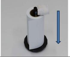
Place paper core on top of black flange so that paper is in a clockwise direction as shown above.
