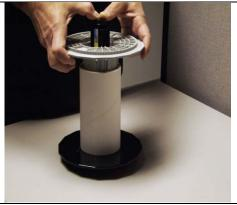
6. Stand the spindle unit on a flat surface with the black spindle down and remove the grey upper flange. The upper flange should always be the gray one.
