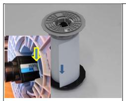
10. Slide the grey flange onto the spindle until fully pushed into the paper core. The number on the Spindle and the Paper Size match (8 inch paper shown)
