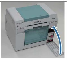
16. Close the cartridge cover and verify the printers  $^{\circlearrowleft}$  light is on.
