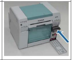
15. Insert the new Maintenance Tank. Push in until the tank locks
