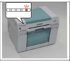
Open cabinet door and check which warning light is lit. The one above indicates the Maintenance Cartridge needs replacement.
