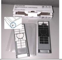
14. Prepare a new Maintenance Cartridge. Be careful not to touch the chip on the new tank.
