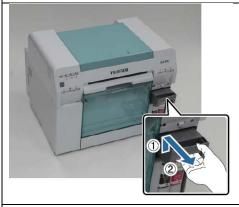
13. To remove gently lift up and then pull out. Be careful not to tilt the cartridge.
