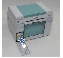
4. Press the ink cartridge requiring replacement lightly to unlock it.
