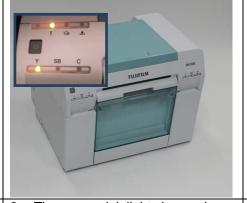
The orange ink light shown above indicates it's necessary to replace an ink cartridge. This example shows a Y (yellow) cartridge.
