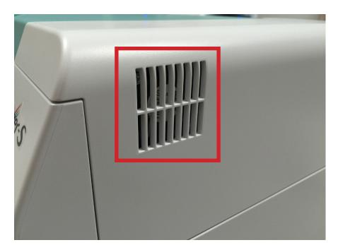
2. Vacuum these louvers, if there is any residual debris wipe it away with a damp bemcot to keep the area clean.
