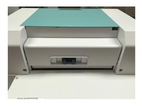
2. Using a bemcot moistened with water place the bemcot on the soft rubber rollers and rotate the shaft by hand. Then close the rear cover.
