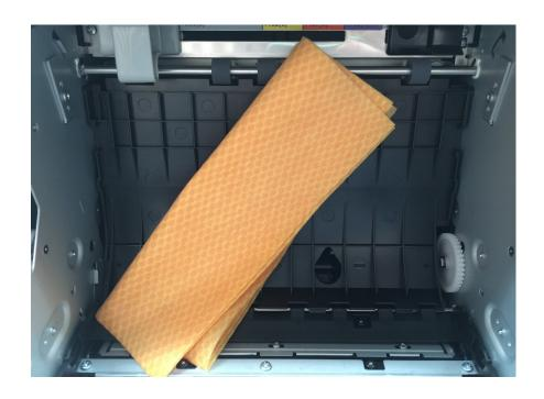
3. Utilizing a list free cloth or a bemcot. Gently wipe the inside of the roll unit to remove any dirt or debris.
