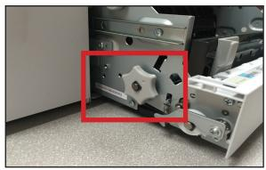
7. Using a bemcot moistened with water. Place the bemcot on each gray roller outlined while turning the gray knob backwards and forwards to ensure
