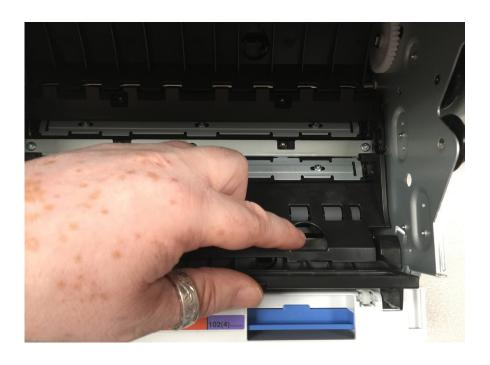
7. Gently wipe this area of any dust or debris. Brush lightly across the felt pads to remove excess paper dust.
