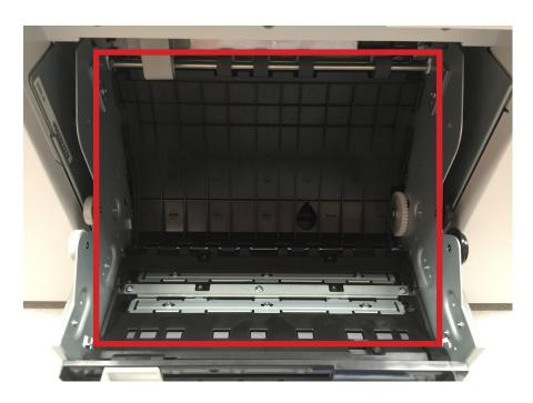
4. Lift up the rear plate by placing your finger in the teardrop hole and lifting upwards.
