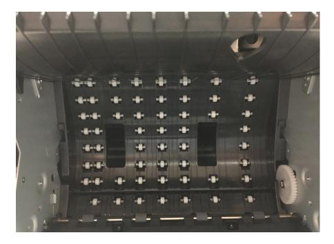
6. Lift up on the front plate, by placing your finger in the hole and lifting upwards
