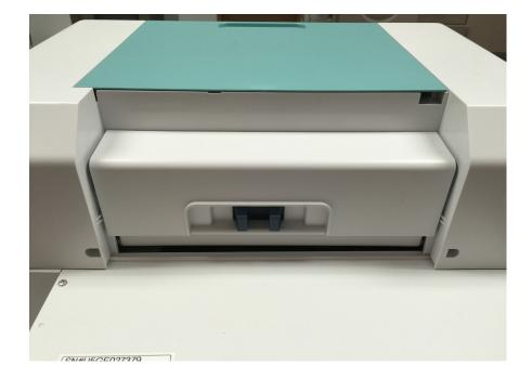
The roll unit is a vital part of the DX100's paper transport section. It is important to maintain this sections cleanliness by follow the steps below.
