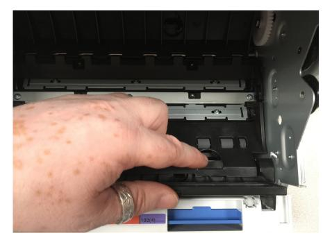
9. Using a bemcot moistened with water. Place the bemcot on each gray roller while turning the gray knob backwards and forwards to ensure
