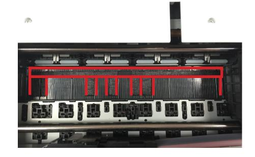
4. Utilizing a lightly moistened bemcot, Wipe any residual ink from the hard plastic platen.
