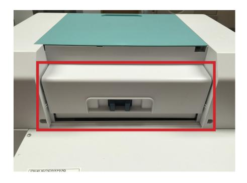
Note: To better clean these rollers it is best to push down on the paper guides to raise the rollers from the main feed roller.
