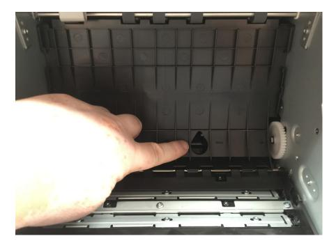
5. Lift up the rear plate by placing your finger in the teardrop hole and lifting upwards.
