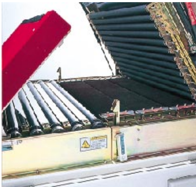
Photo 3 Thermal development parts of FDS-6100X
