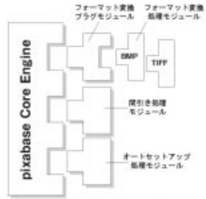
Fig. 4 Image processing architecture of “pixabase”
