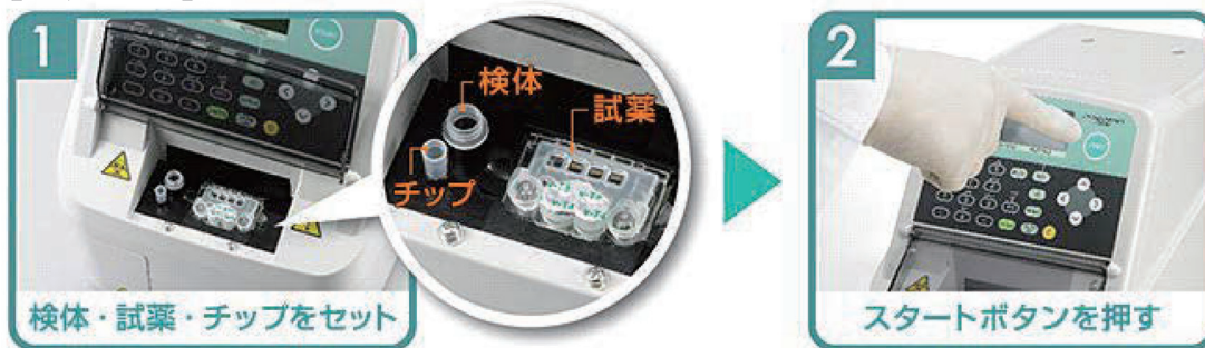
Fig. 2 Quantitative immunoassay system for measuring TBA levels in dog and cat serum and plasma
