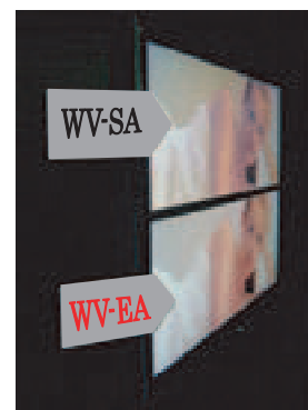
Fig. 10 Dependence of color shift at white state on horizontal viewing angle, and oblique view of WV-SA (upper) and WV-EA (lower).
