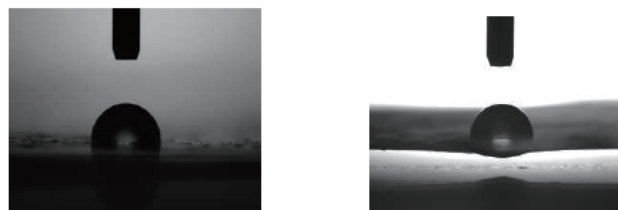
Fig. 8 Comparison of contact angle for polycaprolactone film to H 2 O, (A) Flat film ; (B) "Honeycomb film".
