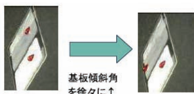
Fig. 9 Image of H 2 O drop grip test for polycaprolactone film. Front side is “Honeycomb film”. Back side is a flat film. Drops are colored by dye for better understanding.
