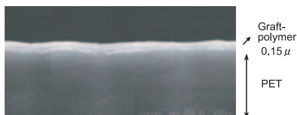
Fig. 2 Cross-sectional view of a PET film photografted with use of acrylic acid.
