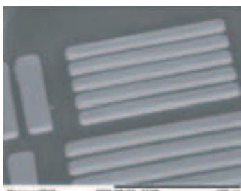
Fig. 5 Copper fine pattern obtained by direct metalization.
