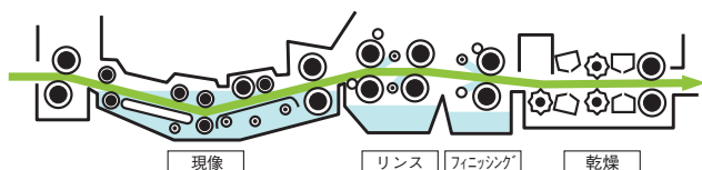
Fig. 1 Developing process of positive thermal CTP plate.
