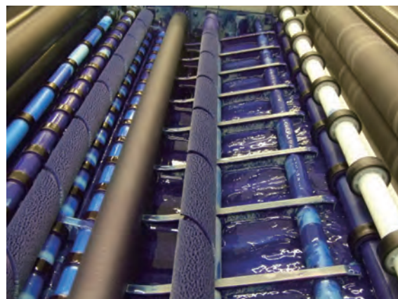
Fig. 3 Precipitation in a present developer tank
