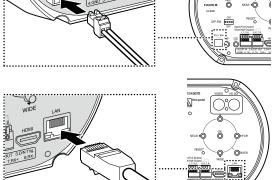
**3** Select IP mode by setting DIP switch ② to "ON" and DIP switches ①, ③ and ④ to "OFF".
