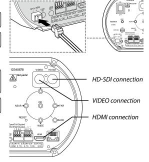
3 Select stand-alone mode by setting DIP switches 1 and 2 to "ON".
