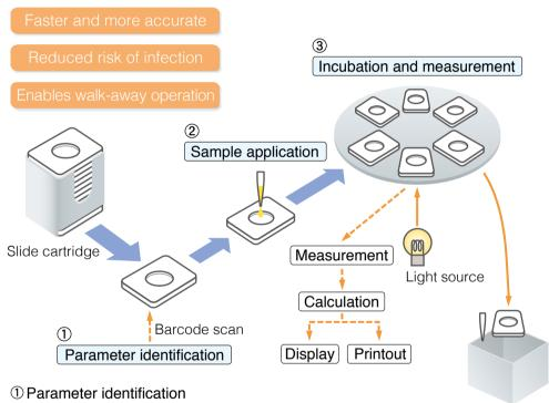
The test parameter and slide lot are identified by the barcode or 2D dot code printed on the back of the slide. (The sample application amount, measurement wavelength, reaction time, and other information are also loaded at the same time.)
