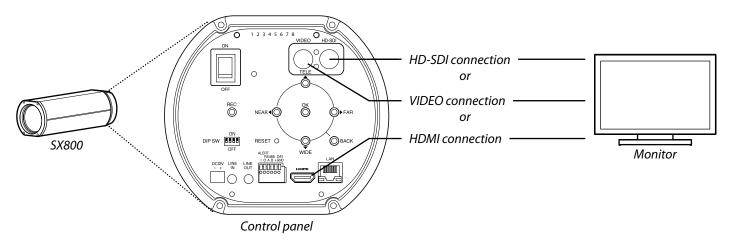
When the camera is connected to a monitor via an HD-SDI, VIDEO, or HDMI cable, you can view the live feed, control the camera, and adjust camera settings via the control panel on the back of the camera.
