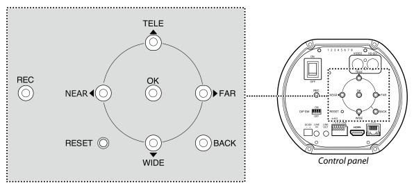
The following buttons are used to navigate the menus and control the camera:
