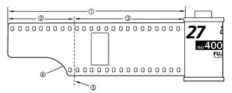
Together, the film extraction length and leading end length should not total more than 4 3/4 in. (120 mm).
