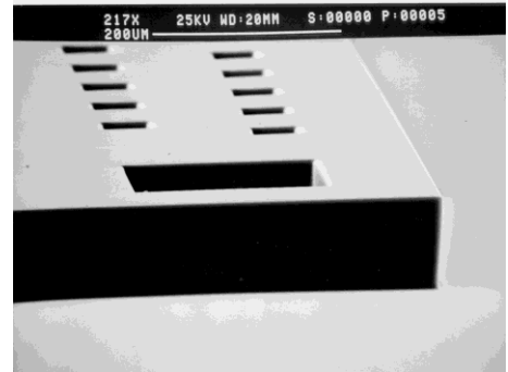
Via mask in 40µm softbake film
