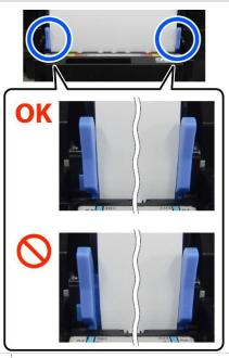
Align the edge guides to the width of the roll paper.
