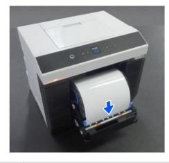
Confirm that there are no gaps between the media edge guide and the roll paper, lower the knob, and then secure the media edge guide.
